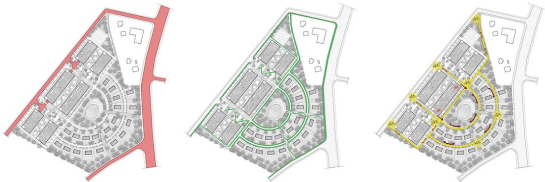
Figure 8. Schemes of motor, pedestrian and bicycle traffic
