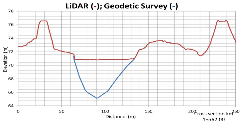
**Fig. 6** Cross-section surveyed with LiDAR technology and the boatborne echo sounder
