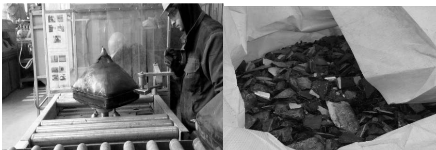
Figure 1. Appearance of automatic separator CRT (left); Glass shards after recycling (right)
