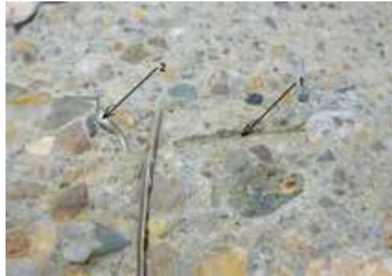
Figure 7. The surface of the concrete sample micro-reinforced with steel fibers ZS/N – 0,50x30mm: 1 – fiber indentation, 2 – fiber cutting
