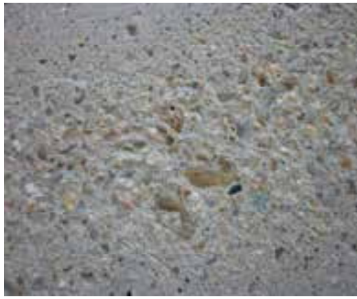
Figure 9. Surface of the sample of concrete micro-reinforced with polypropylene fibers
