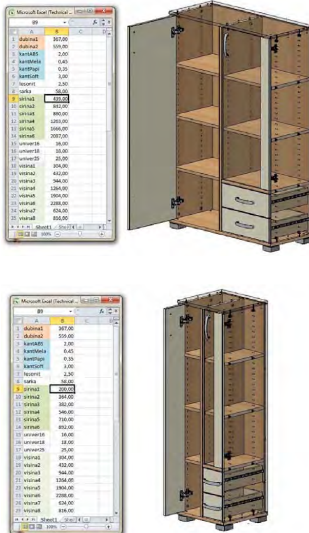
Fig.15. An example: element K22-S defined with parameters given in table – width and depth
