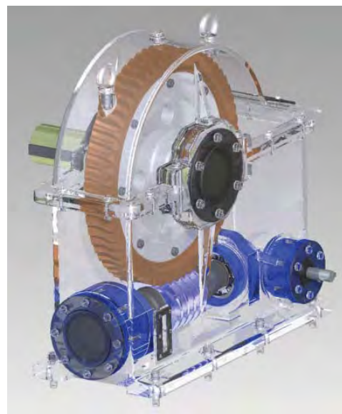
Fig. 6: Combined power transmission - worm gear pair and bevel gear pair
