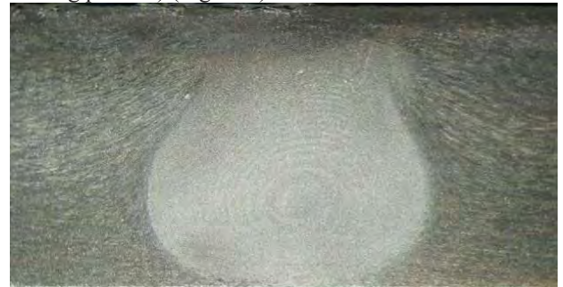
Figure 6 Macroscopic section on nugget zone of the FSW weld on 2024 alloy [2]
