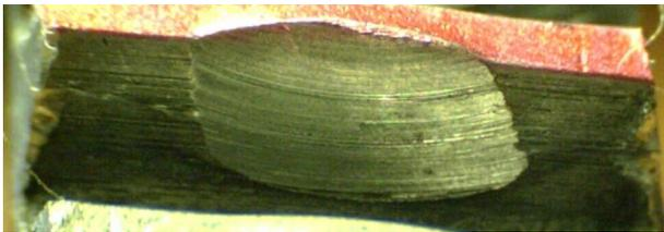
**Figure 4.** Wear on wheel tooth surface without additional treatment for  $T_2 = 36 \text{ Nm}$ ;  $t = 260 \text{ h}$ ;  $n_1 = 5000 \text{ min}^{-1}$
