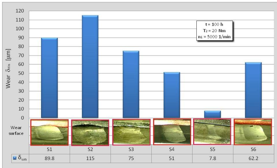
**Figure 5.** Wear  $\delta_{wn}$  for all trials with different material variants [6]
