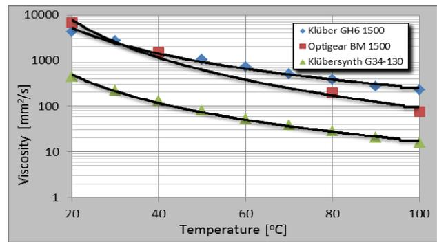
**Figure 2.** Viscosity-temperature behaviour for used lubricants
