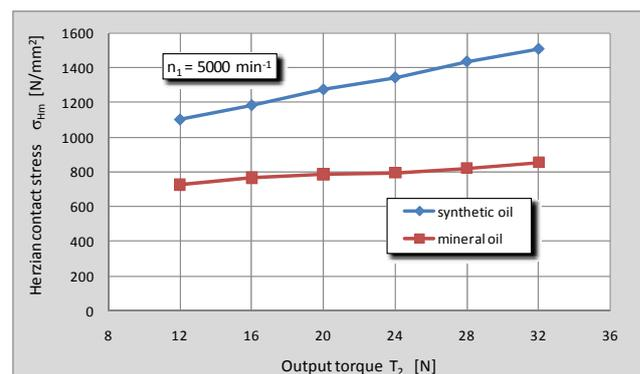
**Figure 3.** Hertzian contact stress  $\sigma_{Hm}$  for duration of the experiment with different lubrication and  $n_1 = 1500; 5000$  and  $10000 \text{ min}^{-1}$
