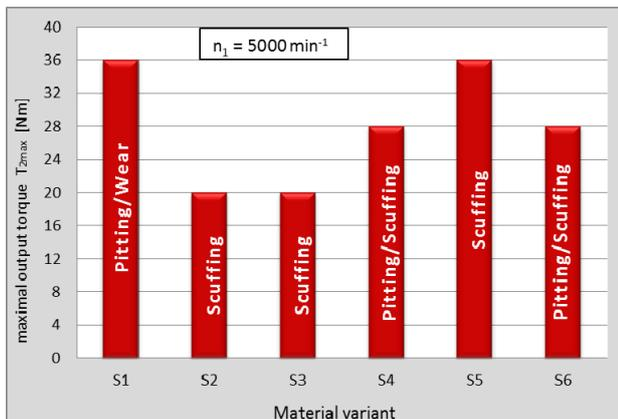
**Figure 8.** Comparison of maximum transmissible torque with critical damage type for different materials and input speed  $n_1 = 5000 \text{ min}^{-1}$  [8]
